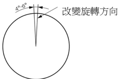
一般情況下這意味著:  $\dot{\alpha}_{Mot} = 5^\circ/s = 5^\circ \times 60/min = 300^\circ/min = 300/360 \text{ rpm} = 0.83 \text{ rpm}$
