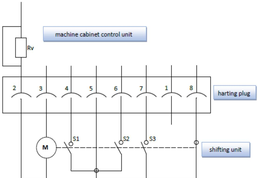
wiring diagram for switch over gear 1>2
