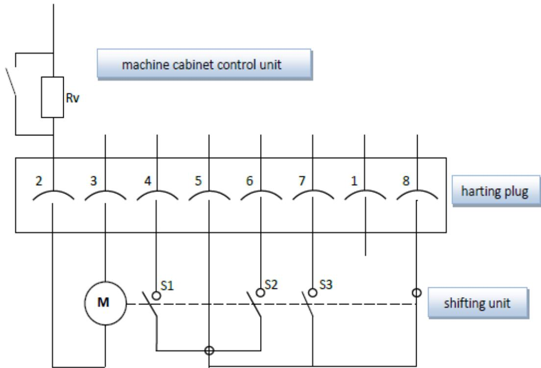
wiring diagram for switch over gear 1 > N-position or gear 2 > gear1 > N-position
